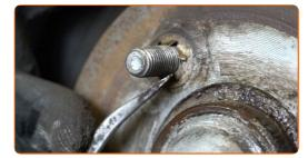
18 Remove the brake disc.
