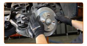
Screw in the brake disc fastener. Use a crowbar.
