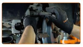
Tighten the brake caliper bracket. Use a drive socket #13. Use a torque wrench. Tighten it to 55 nm torque.
