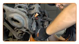
Remove the caliper bracket.
