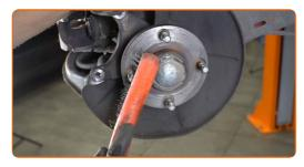
20 Install the brake disc.
