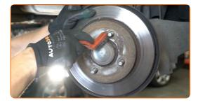
Unscrew the brake disc fastening. Use a crowbar.
