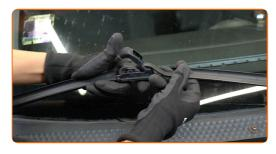
Remove the blade from the wiper arm.
