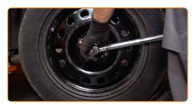
Tighten the wheel bolts using a criss-cross pattern. Use wheel impact socket #19. Use a torque wrench. Tighten it to 110 Nm torque.
