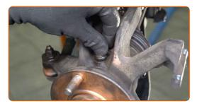
Tighten the fastener that connects the ABS sensor to the steering knuckle. Use a drive socket #8. Use a torque wrench. Tighten it to 5 Nm torque.
