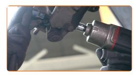
Remove the fastening bolt.
