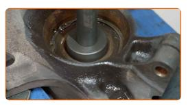
Pull the bearing inner race out of the wheel hub. Use a bearing separator. Use a bush and bearing driver set.
