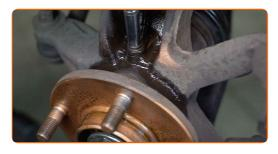
Disconnect the ABS sensor. Use a crowbar.
