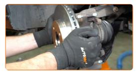
Clean the ABS sensor mounting seat. Use a wire brush. Use WD-40 spray.
