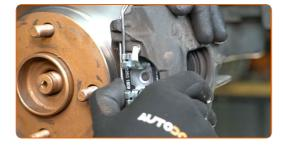
Tighten the brake caliper fasteners. Use HEX No.H7. Use a torque wrench. Tighten it to 28 Nm torque.
