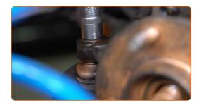
Tighten the fastening nut connecting the tie rod end to the steering knuckle. Use a drive socket #15. Use a torque wrench. Tighten it to 47 Nm torque.
