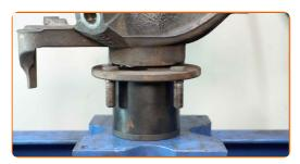
Install the wheel hub bearing retaining ring. Use circlip pliers.
