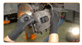
Install the brake caliper retaining spring.
