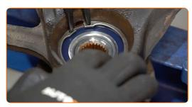
Treat the shock strut mounting seat on the steering knuckle. Use a wire brush. Use WD-40 spray.
