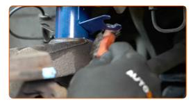
Unscrew the fasteners connecting the suspension strut to the steering knuckle. Use a drive socket #15. Use a tap wrench. Use a ratchet wrench.
