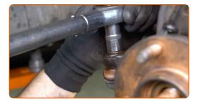
Treat the ABS sensor fastener. Use a multipurpose grease. Use a flat screwdriver.
