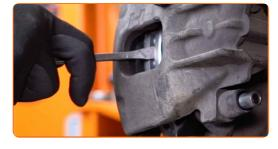
Remove the brake caliper.
