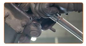
Tighten the lower fasteners connecting the shock strut to the steering knuckle. Use a drive socket #15. Use a torque wrench. Tighten it to 90 Nm torque.
