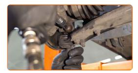
Tighten the fastener connecting the ball joint to the steering knuckle. Use a drive socket #15. Use a torque wrench. Tighten it to 47 Nm torque.
