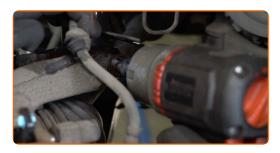
Remove the fastening bolt.
