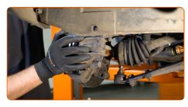
Clean the ball joint mounting seat. Use a wire brush. Use WD-40 spray.
