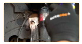
Unscrew the fastener connecting the stabilizer link to the shock strut. Use a combination spanner #15. Use a drive socket #15. Use a ratchet wrench.
