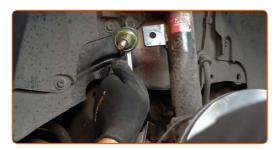
Detach the brake hose from the shock strut. Use a crowbar.
