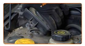
Clean the fasteners of the shock absorber upper mount. Use a wire brush. Use WD-40 spray.
