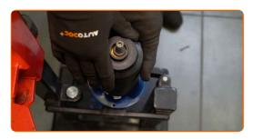
Install the spring on the shock absorber.
