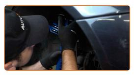
Secure the upper fasteners of the shock strut (3 pieces). Do not tighten it.
