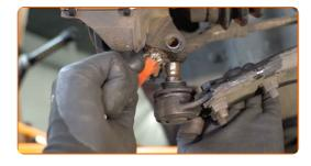
63 Connect the ball joint to the steering knuckle.
