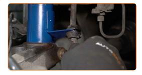
75 Treat the shock strut fasteners. Use copper grease.
