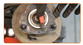
Remove the strut piston rod nut. Use a drive socket #19. Use HEX No.H6. Use a ratchet wrench.
