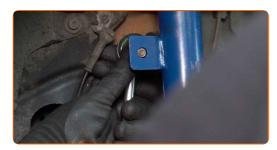
Tighten the stabiliser link fastener. Use a combination spanner #15. Use a drive socket #15. Use a ratchet wrench.
