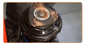
Remove the assembled shock strut.
