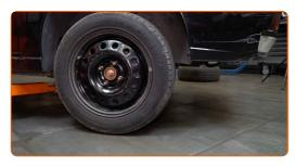
Tighten the drive shaft nut. Use a drive socket #32. Use a torque wrench. Tighten it to 275 Nm torque.
