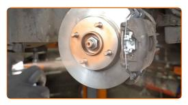
78 Clean the brake disk surface. Use a brake cleaner.
