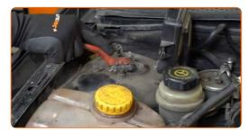
Loosen the upper fasteners of the suspension strut (3 pieces). Use a drive socket #13. Use a ratchet wrench.
