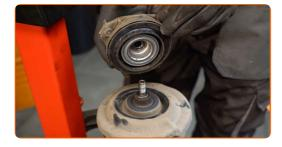
Release the coil spring.
