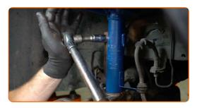
Fasten the brake hose on the strut.
