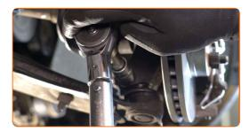
Tighten the lower fastening of the shock absorber. Use a drive socket #15. Use a torque wrench. Tighten it to 90 Nm torque.
