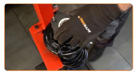
Tighten the shock strut piston rod nut. Use a drive socket #19. Use HEX No.H7. Use a torque wrench. Tighten it to 48 Nm torque.
