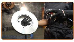
19 Install the brake disc.
