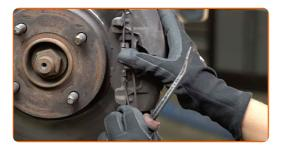
Remove the brake caliper.
