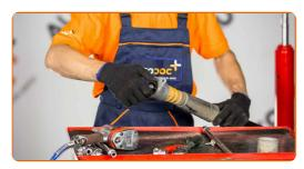
Tighten the shock absorber mount fasteners. Use a drive socket #13. Use a torque wrench. Tighten it to 25 nm torque.
