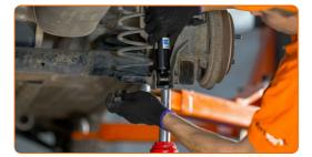
Tighten the lower fastener of the shock absorber. Use a drive socket #15. Use a torque wrench. Tighten it to 115 Nm torque.
