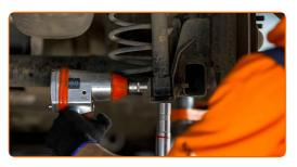
9 Remove the fastening bolt.
