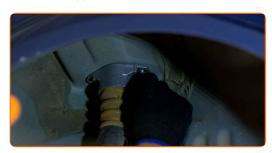
Tighten the top shock absorber fastening. Use a drive socket #10. Use a torque wrench. Tighten it to 25 Nm torque.
