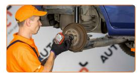
10 Remove the brake drum.
