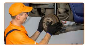
Tighten the fastener of the wheel hub bearing. Use a drive socket #30. Use a torque wrench. Tighten it to 235 Nm torque.
