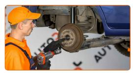
Unscrew the hub bearing mounting. Use a drive socket #30.
