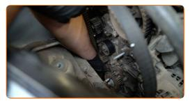
Remove the timing belt tensioner pulley.
