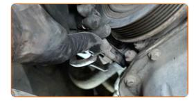
130 Attach the crankshaft position sensor wiring.
