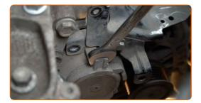
Screw in the fastener of the serpentine belt tensioner pulley. Use a drive socket #10. Use a ratchet wrench.
