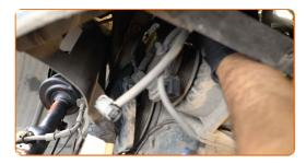
126 Attach the alternator wiring harness.
