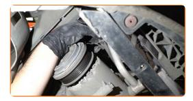
Disconnect the alternator connector.
