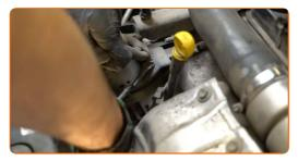
Disconnect the engine wiring harness connector.
