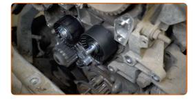
Tighten the fastener of the timing belt idler pulley. Use a drive socket #16. Use a torque wrench. Tighten it to 37 Nm torque.
