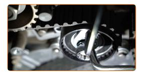
Remove the timing belt tensioner pulley locking tool.
