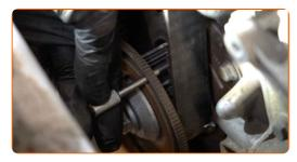
Turn the crankshaft pulley. Use a drive socket #18. Use a ratchet wrench.
