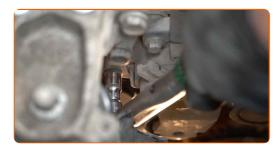
Install the coolant reservoir. Make sure you hear a click indicating that it is locked in place.
