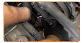
Pull aside the timing belt tensioner pulley.
