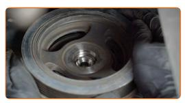
Tighten the crankshaft pulley fastener. Use a drive socket #18. Use a torque wrench. Tighten it to 35 Nm torque.+190°
