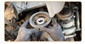
Unscrew the fasteners of the lower timing cover. Use a drive socket #7. Use a ratchet wrench.
