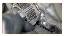
Unscrew the fastener of the timing belt idler pulley. Use a combination spanner #16.
