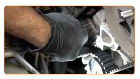
Remove the crankshaft gear locking tool.
