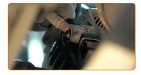
Detach the alternator wiring harness clip from the bracket. Use a clip removal tool.
