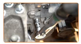
Tighten the fastener of the serpentine belt tensioner pulley. Use a drive socket #10. Use a torque wrench. Tighten it to 16 Nm torque.
