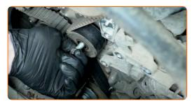
Remove the timing belt idler pulley from its mounting seat.
