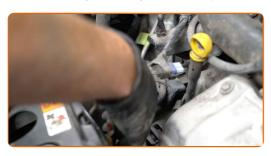
Attach the alternator wiring harness clip to the bracket.
