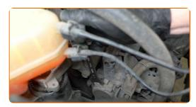
Disconnect the connector of the air conditioner compressor.
