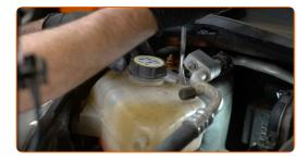
Remove the coolant reservoir.
