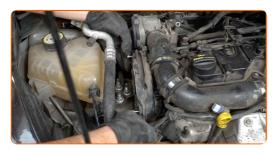
Screw in the fasteners of the upper timing cover. Use a drive socket #7. Use a ratchet wrench.
