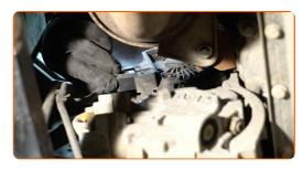
Connect the alternator connector.
