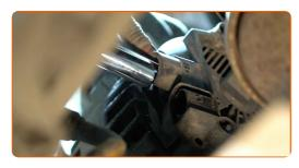
Detach the alternator wiring harness.
