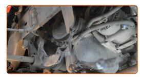
Unscrew the fasteners of the engine wiring harness bracket. Use a drive socket #8. Use a ratchet wrench.
