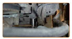
Detach the engine wiring harness clip from the timing cover. Use a clip removal tool.
