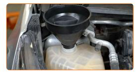
Pour coolant in the coolant reservoir.
