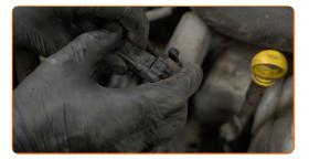
Connect the engine wiring harness connector.
