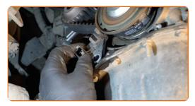
Tighten the fastener of the crankshaft position sensor. Use a drive socket #8. Use a torque wrench. Tighten it to 9 Nm torque.
