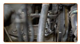
Tighten the upper fastener of the engine mount. Use a drive socket #15. Use a torque wrench. Tighten it to 50 Nm torque.
