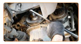
Remove the crankshaft pulley.
