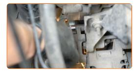
Remove the serpentine belt tensioner pulley.
