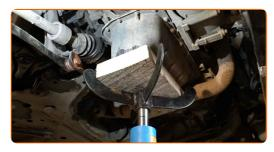
Clean the engine mount fasteners. Use WD-40 spray.
