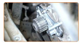
Tighten the water pump fasteners. Use a drive socket #8. Use a torque wrench. Tighten it to 10 Nm torque.
