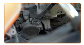
Unscrew the fasteners of the alternator wiring harness bracket. Use a drive socket #10. Use a ratchet wrench.
