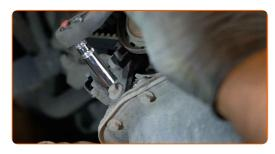
Remove the crankshaft position sensor.
