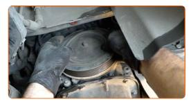
Screw in the fasteners of the engine wiring harness bracket. Use a drive socket #8. Use a ratchet wrench.
