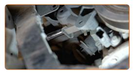
Remove the crankshaft pulley cap. Use a flat screwdriver.
