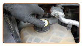
Screw on the coolant reservoir cap.
