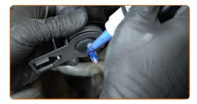
Install the timing belt tensioner pulley.
