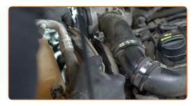
Unscrew the fasteners of the lower serpentine belt cover. Use Torx T30. Use a ratchet wrench.
