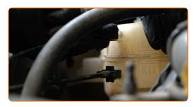
Clean the lower coolant pipe mounting seat. Use all-purpose cleaning spray.
