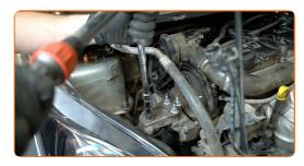
97 Remove the support from under the engine.
