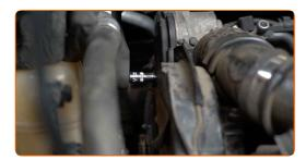
Attach the engine wiring harness to the upper timing cover.
