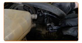
Detach the clamp of the lower coolant pipe. Use combination pliers.
