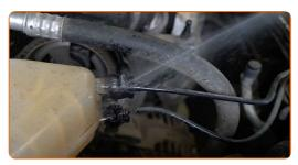
Detach the coolant hoses from the coolant reservoir.
