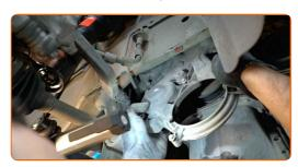
Unscrew the fastener of the crankshaft position sensor. Use a drive socket #8. Use a ratchet wrench.
