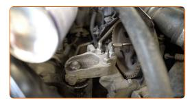
Unscrew the upper fastener of the engine mount. Use a drive socket #15. Use a ratchet wrench.
