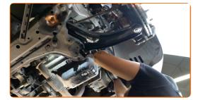
Screw in the alternator wiring harness fastener. Use a drive socket #13. Use a ratchet wrench.
