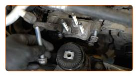
Tighten the engine mount fastening bolts. Use a drive socket #16. Use a torque wrench. Tighten it to 55 Nm torque.
