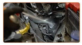
Unscrew the filter housing cap together with the old filter element. Use a drive socket #27. Use a ratchet wrench.
