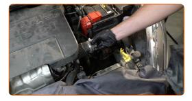
Reinstall the air filter housing.
