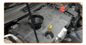
Pour oil into the engine through the filler. Required amount of oil: 4 l.
