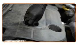
Tighten the oil filler cap.
