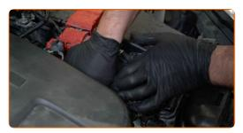
Remove the air filter housing.
