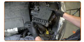
Cover the air intake hose with a microfibre towel to prevent dust and dirt from getting into the system.
