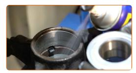
Press the new bearing in the steering knuckle.
