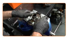
Pull the bearing inner race out of the wheel hub. Use a bearing separator. Use a pin punch. Use a hammer.
