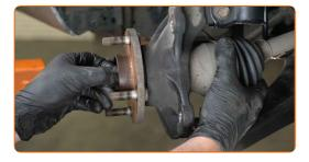
Detach the driveshaft from the steering knuckle.
