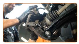
Tighten the brake caliper bracket. Use a drive socket #15. Use a torque wrench. Tighten it to 70 Nm torque.
