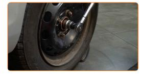
Tighten the wheel bolts using a criss-cross pattern. Use wheel impact socket #19. Use a torque wrench. Tighten it to 110 Nm torque.
