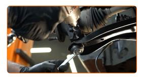
Remove the fastening bolt.
