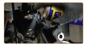
Unscrew the lower fastener connecting the shock strut to the steering knuckle. Use a combination spanner #15. Use a drive socket #18. Use a ratchet wrench.
