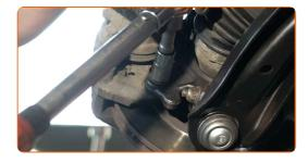
Fasten the brake hose on the strut.
