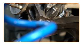
Tighten the lower fasteners connecting the shock strut to the steering knuckle. Use a combination spanner #15. Use a drive socket #18. Use a torque wrench. Tighten it to 82 Nm torque.+90°
