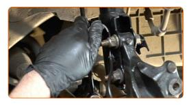
63 Attach the ABS sensor connector.
