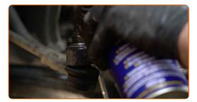
Unscrew the end fastening nut to the steering knuckle. Use a drive socket #18. Use a ratchet wrench.
