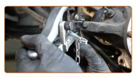
Disconnect the ball joint from the steering knuckle.
