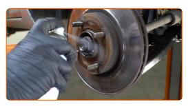
Remove the brake disc.
