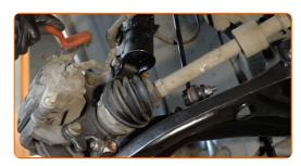
Unscrew the brake caliper fastening. Use a combination spanner #12.
