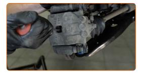
10 Remove the brake caliper.
