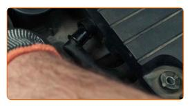
Remove the air intake pipe.
