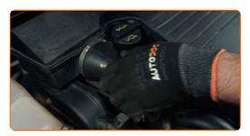
Fasten the clamp on the air intake hose. Use clic-R collar pliers.
