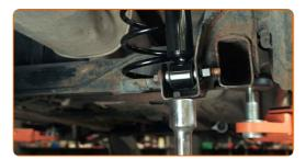
Tighten the lower fastener of the shock absorber. Use a drive socket #15. Use a torque wrench. Tighten it to 115 Nm torque.
