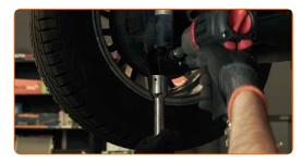
14 Remove the fastening bolt.
