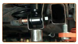
Screw in the lower fastener of the shock absorber. Use a drive socket #15. Use a ratchet wrench.
