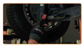
Unscrew the lower fastener of the shock absorber. Use a drive socket #15. Use a tap wrench.
