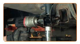
9 Remove the fastening bolt.
