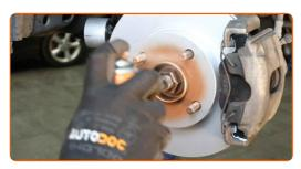
Clean the brake disk surface. Use a brake cleaner. 30
