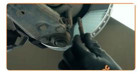
Unscrew the rear fastener connecting the control arm to the subframe. Use a drive socket #13. Use a drive socket #18. Use a tap wrench.
