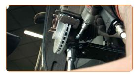
Screw the front arm fastener. Use a combination spanner #18. Use a drive socket #15. Use a tap wrench.
