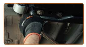
Tighten the rear fastener of the control arm. Use a drive socket #18. Use a torque wrench. Tighten it to 80 Nm torque.+55°
