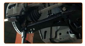
Screw the fasteners of the ball joint. Use a drive socket #15. Use Torx T50. Use a ratchet wrench.
