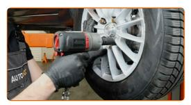
Lower the car and working in a cross order, tighten the wheel bolts. Use wheel impact socket #19. Use a torque wrench. Tighten it to 95 nm torque.
