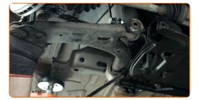
Clean the mounting seats and the thread of the suspension arm. Use a wire brush. Use WD-40 spray.
