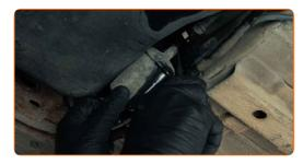
Disconnect the fuel supply lines from the fuel filter. Use fuel line pliers.
