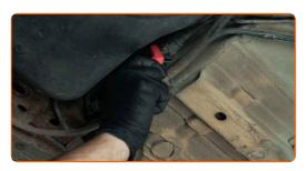
6 Remove the fuel filter. Use a crowbar.
