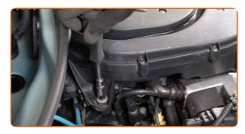
Remove the air filter housing retaining spring.
