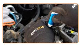
Install the spark plug wire connectors into the spark plug wells. Make sure you hear a click indicating that it is locked in place.
