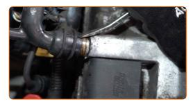
Detach the throttle valve connectors. Use a crowbar.
