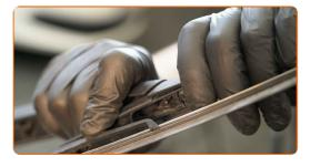
Remove the blade from the wiper arm.
