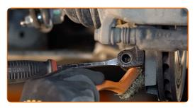
18 Install a new arm. Use a pin punch.
