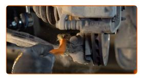
Unscrew the ball joint fastening to the steering knuckle. Use a combination spanner #17. Use a drive socket #17. Use a ratchet wrench.
