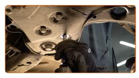
Release the fastener connecting the ball joint to the steering knuckle. Use a crowbar. Use a hammer.
