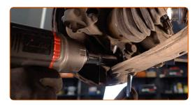
10 Remove the fastening bolt.
