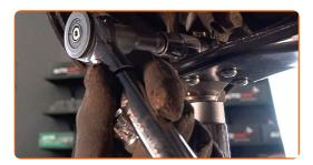
Tighten the front fastener connecting the control arm to the subframe. Use a drive socket #21. Use a torque wrench. Tighten it to 95 Nm torque.+90°
