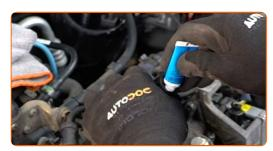
Install the spark plug wire connectors into the spark plug wells. Make sure you hear a click indicating that it is locked in place.
