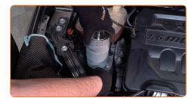
7 Detach the fuel pressure sensor connector.
