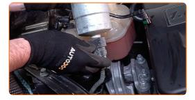
Attach the fuel pressure sensor connector.
