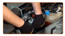
Tighten the fuel filter fasteners. Use a drive socket #10. Use a ratchet wrench.
