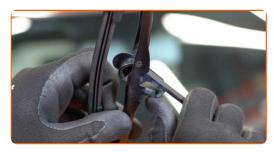
Remove the blade from the wiper arm.
