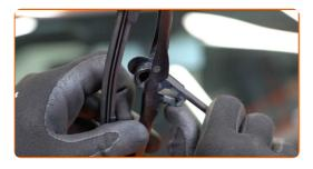
Remove the blade from the wiper arm.
