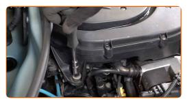
Remove the air filter housing retaining spring.
