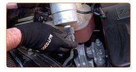
Attach the fuel pressure sensor connector.
