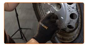
Lower the car and working in a cross order, tighten the wheel bolts. Use a torque wrench. Tighten it to 98 Nm torque.
