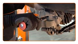
Remove the brake caliper.
