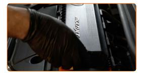
Screw in the fastening screws of the air filter cover. Use a drive socket #7. Use a ratchet wrench.
