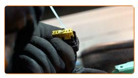
Attach the fuel pressure sensor connector.
