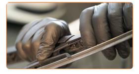
Remove the blade from the wiper arm.
