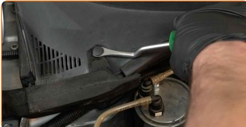
4 Unscrew the fasteners of the cowl grille. Use a Phillips screwdriver.
