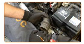
Undo the fastening screws of the air filter cover. Use a drive socket #10. Use a ratchet wrench.
