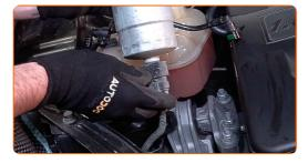
Attach the fuel pressure sensor connector.
