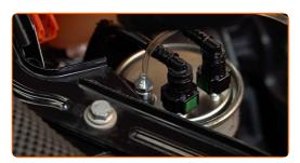
Unscrew the fuel filter bleeder screw. Use a combination spanner #12.
