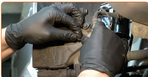
**30** Treat the surface where the brake disc contacts the wheel rim. Use copper grease.
