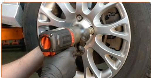
**34** Lower the car and working in a cross order, tighten the wheel bolts. Use wheel impact socket #17. Use a torque wrench. Tighten it to 120 Nm torque.
