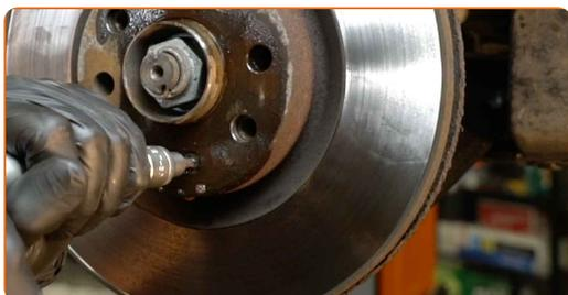
**18** Remove the brake disc.
