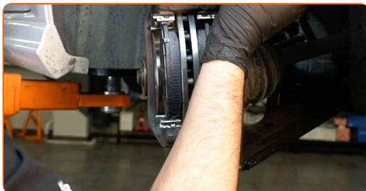
**28** Install the brake caliper and fix it. Use a drive socket #13. Use a torque wrench. Tighten it to 30 Nm torque.
