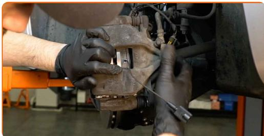
**29** Connect the brake pads wear sensor.
