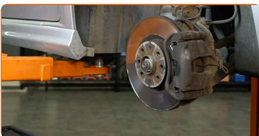
**7** Disconnect the brake pads wear sensor.
