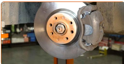
**31** Clean the brake disc surface. Use a brake cleaner.
