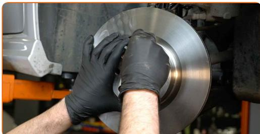
**21** Tighten the brake disc fastening. Use Torx T30. Use a torque wrench. Tighten it to 9 Nm torque.
