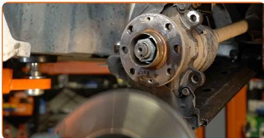
**19** Clean the hub. Use a wire brush. Treat the contacting surface. Use copper grease.
