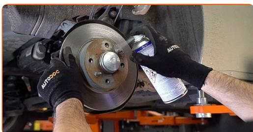
**15** Unscrew the brake disc fastening. Use a drive socket #12. Use a ratchet wrench.
