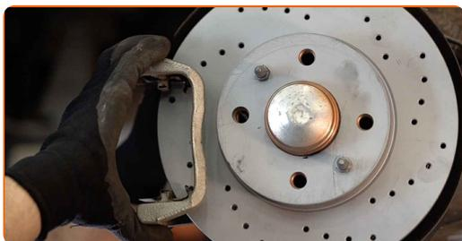
**21** Tighten the brake caliper bracket. Use a combination spanner #13. Use a torque wrench. Tighten it to 54 Nm torque.
