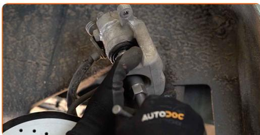
**26** Install the brake caliper and fix it. Use a combination spanner #17. Use a drive socket #13. Use a ratchet wrench. Use a torque wrench. Tighten it to 27 Nm torque.
