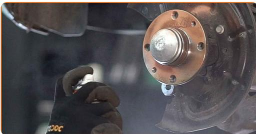
**18** Install the brake disc.
