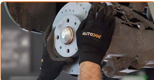
**19** Tighten the brake disc fastening. Use a drive socket #12. Use a torque wrench. Tighten it to 9 Nm torque.
