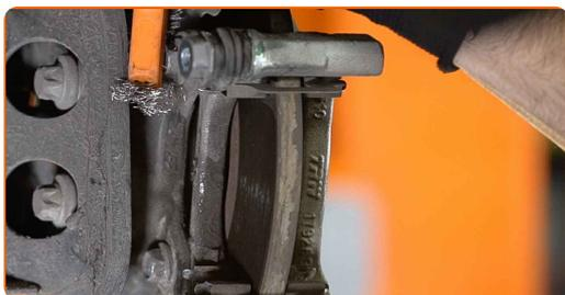
**12** Unscrew the caliper bracket fastening. Use a combination spanner #13.
