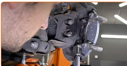
**22** Clean the brake caliper bracket from dirt and dust. Use a wire brush. Use a brake cleaner.
