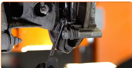
**13** Remove the caliper bracket.
