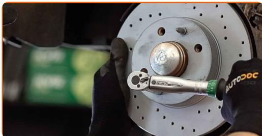
**20** Install the brake caliper bracket.
