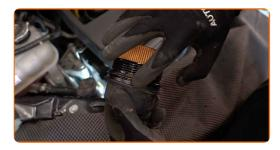
Screw the new filter into its place.
