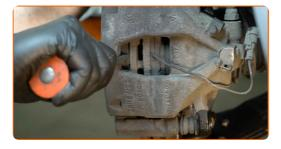
11 Remove the brake caliper.
