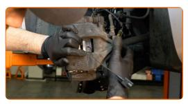
Connect the brake pads wear sensor.
