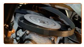
Return the tensioner pulley to its initial position. Use a combination spanner #15.
