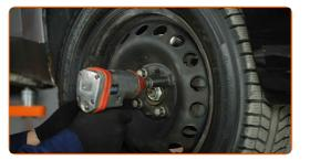
38 Lower the car and working in a cross order, tighten the wheel bolts. Use a torque wrench. Tighten it to 98 Nm torque.
