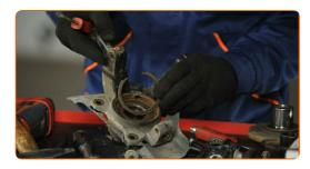
Press out the wheel hub bearing.
