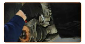
Install the ABS sensor on the steering knuckle and secure it. Use a drive socket #10.
