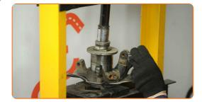
Tighten the lower fasteners connecting the shock strut to the steering knuckle. Use a combination spanner #17. Use a drive socket #17. Use a torque wrench. Tighten it to 75 Nm torque.
