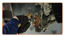
Install the brake disc and secure it. Use a drive socket #12.
