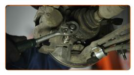
Connect the brake hose fastener to the shock absorber strut.
