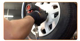
Lower the car and working in a cross order, tighten the wheel bolts. Use a torque wrench. Tighten it to 86 nm torque.
