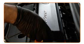
Screw in the fastening screws of the air filter cover. Use a drive socket #7. Use a ratchet wrench.
