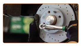
20 Install the brake caliper bracket.
