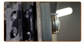
Clean the brake disk surface. Use a wire brush. Use WD-40 spray.
