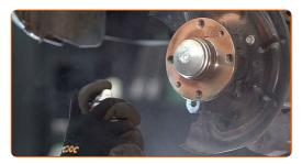
18 Install the brake disc.
