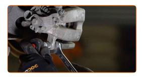
g Remove the brake caliper.
