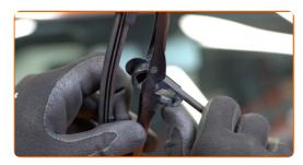
Remove the blade from the wiper arm.
