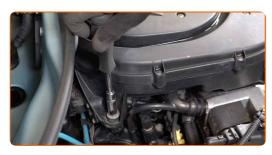
Remove the air filter housing retaining spring.
