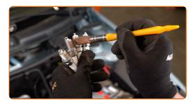
Install the new spark plugs into their mounting seats. Use the spark plug socket #16.
