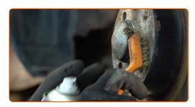
Unscrew the brake disc fastening. Use a drive socket #12. Use a ratchet wrench.
