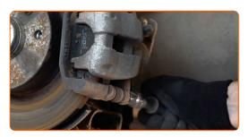
Remove the brake caliper. Use a crowbar.
