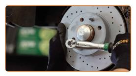
20 Install the brake caliper bracket.
