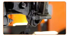
Remove the caliper bracket.
