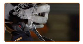
g Remove the brake caliper.
