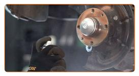
18 Install the brake disc.
