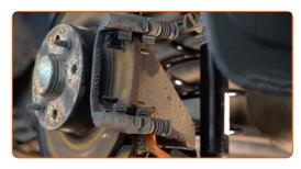
Unscrew the caliper bracket fastening. Use a drive socket #17. Use a tap wrench.
