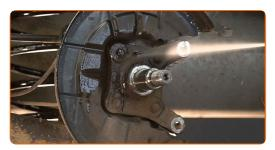
20 Install the new wheel hub with a bearing.
