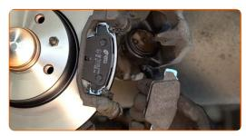
Install the brake caliper and fix it. Use a drive socket #13. Use a torque wrench. Tighten it to 30 Nm torque.
