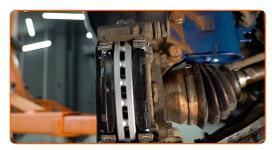
Install the brake caliper and fix it. Use a drive socket #13. Use a torque wrench. Tighten it to 27 Nm torque.
