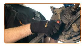
Remove the caliper bracket.
